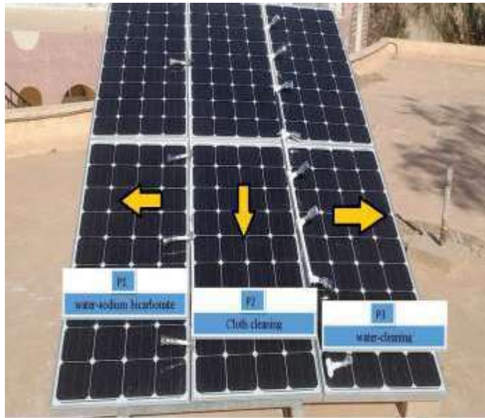
Figure 1. Experimental test bench (URAER)
