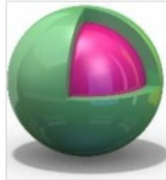
Figure 2. Model of a micro-encapsulated PCM with a wax core and polymer capsule [19].
